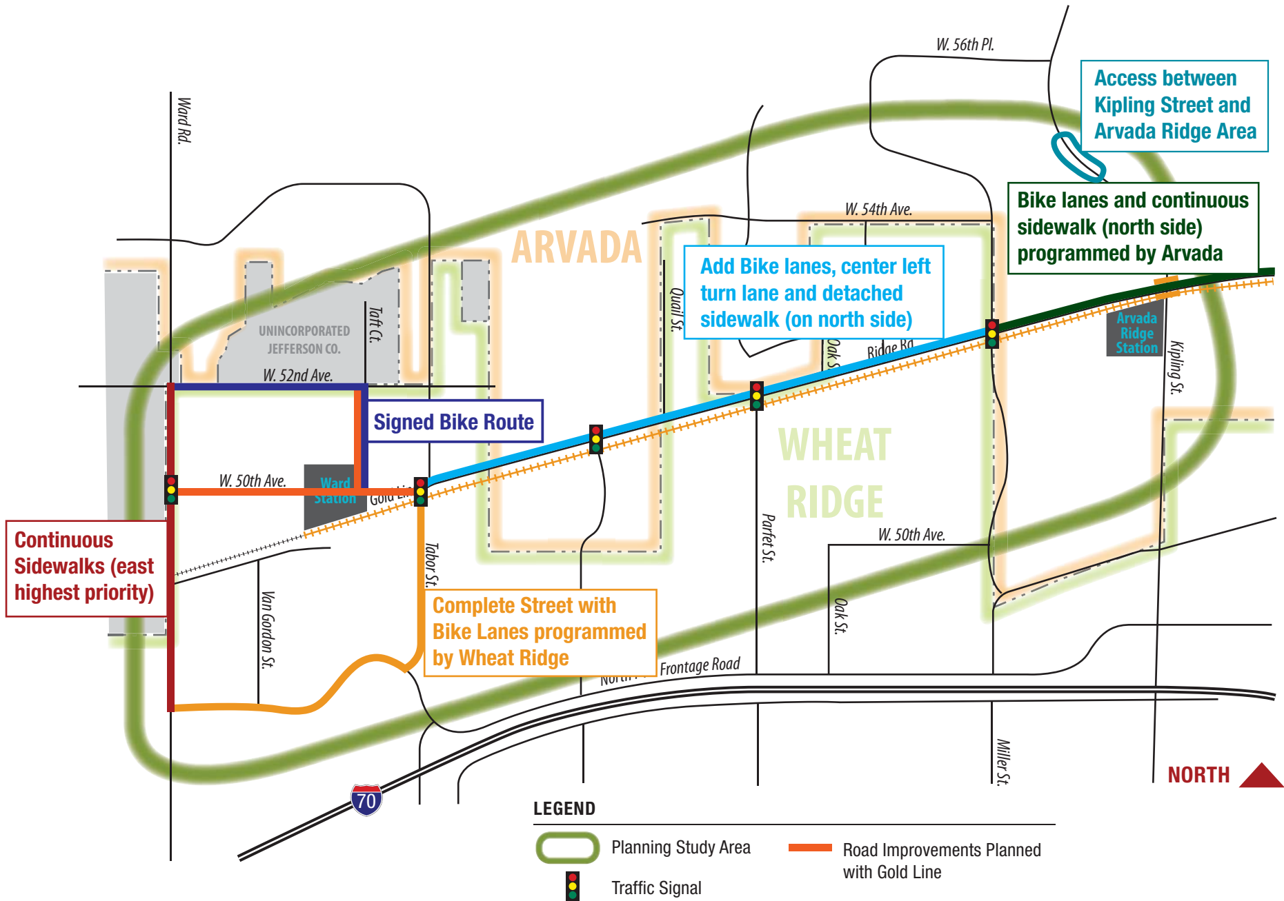
Figure 1 Recommended Access Improvements
