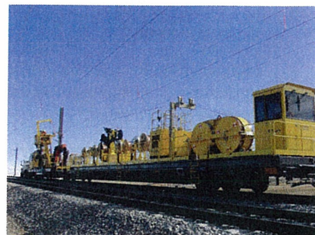
The Wire Train installs overhead wire on the East Rail Line.
