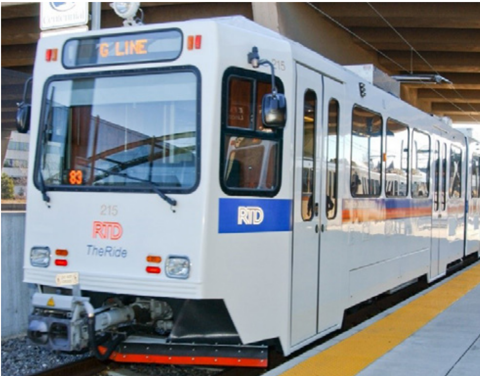
Figure 11: Light Rail Vehicle (Siemens SD-160)
