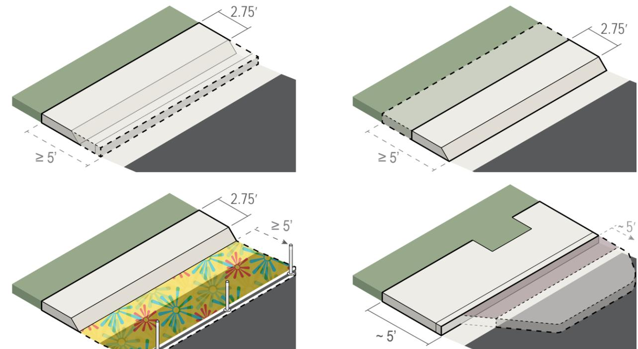
**Figure 26** Four typical solutions to expanding substandard sidewalks. Clockwise from top left: extending the curb into the road to achieve standard width; extending the sidewalk back toward the property line; using "paint-and-post" interim materials to extend into the road; and bulb-outs to navigate obstructions.
