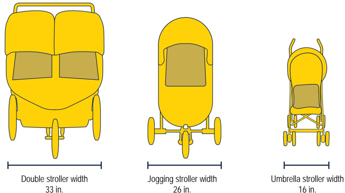
Figure 2 Stroller Dimensions and Pedestrian Space Requirements (Source: Alta Planning + Design)
