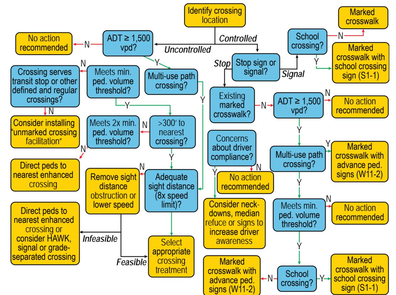
Figure 15 Boulder Uncontrolled Pedestrian Crossing Treatment Flowchart
