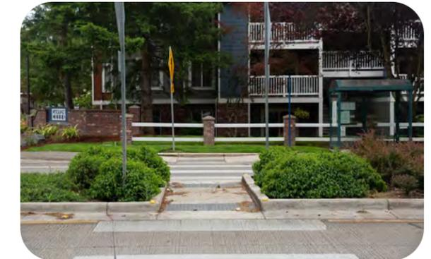
Figure 23 Pedestrian island and median. (Source: Alta Planning + Design)
