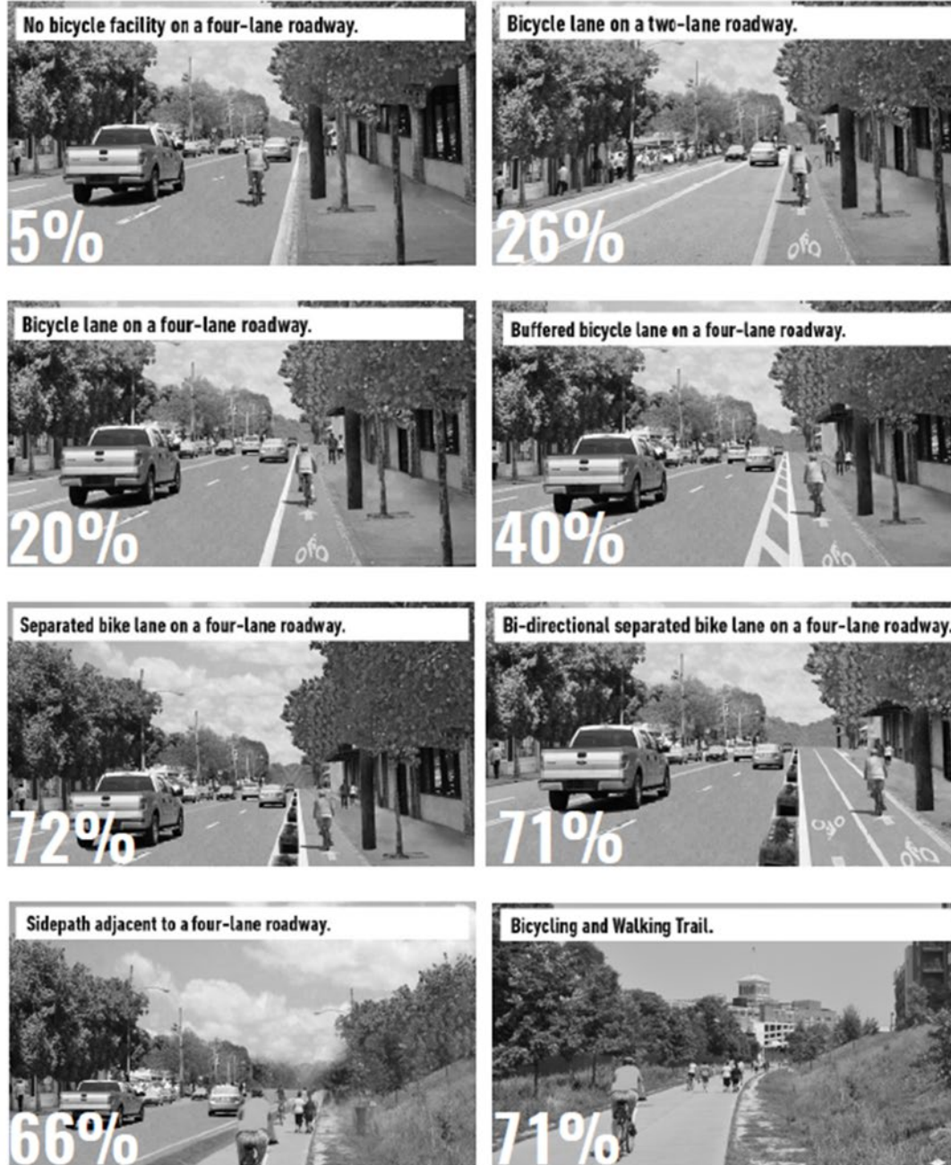
Figure 11. Denver region residents who said they would feel comfortable by bicycle facility type.
