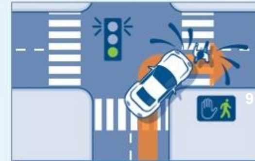
Right Turn Pedestrian Crash at Signalized Intersections
