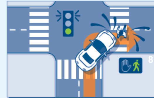
Right Turn Pedestrian Crash at Signalized Intersections
