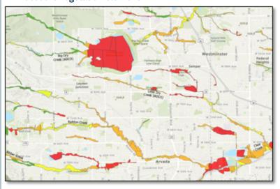
As another example, the land development intensity index is derived from DRCOG's land cover dataset and contributes to the scoring of the hydrology element. Figure 2 shows minimal to significant development on a scale from green to red.
